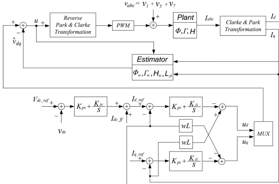
Figure 6. Block diagram of the observer-based control configuration including input current harmonic compensation.
