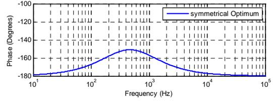
Figure 8. Bode diagram of the current controller based on the Symmetrical Optimum (SO) method (5 kHz).
