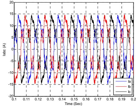
Figure 11. Simulated input current waveforms without observers resulting in 31.3% THD harmonic content.
