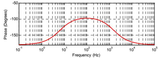
Figure 10. Bode diagram of the dc link voltage controller based on pole-zero cancellation method (5 kHz sampling).
