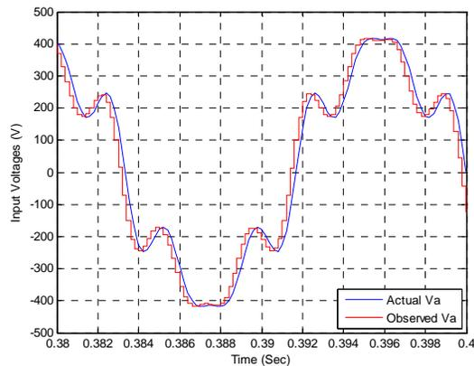
Figure 13. Zoomed-in view of simulated phase-A input voltage and the observed input voltage (5 kHz sampling).
