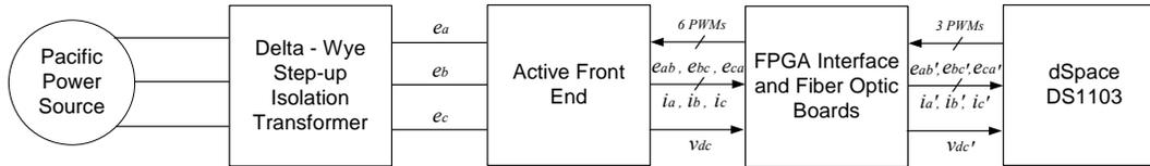
Figure 15. Block diagram of experimental test configuration.
