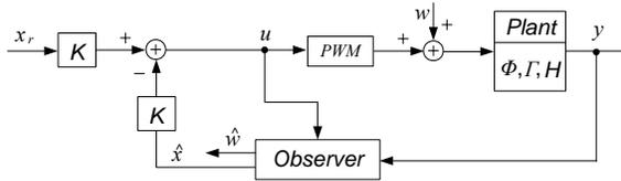
Figure 3. System block diagram including the disturbance  $w$  and closed-loop disturbance observer.
