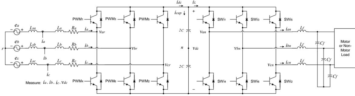
Figure 1. Four-quadrant ASD or UPS with active front-end (AFE) voltage source converter (VSC).
