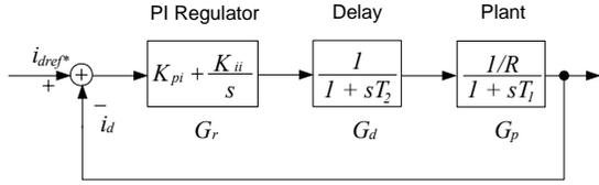
Figure 7. Block diagram of the closed-loop current regulator with PI controller.
