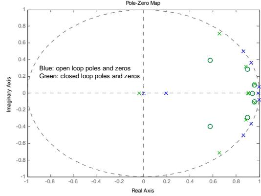
Figure 5. Controller pole-zero diagram in complex  $z$ -plane including the 5<sup>th</sup> and 7<sup>th</sup> harmonics observers (5 kHz sampling).
