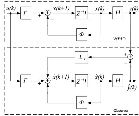
Figure 2. Block diagram of closed-loop observer system in discrete  $z$ -domain.
