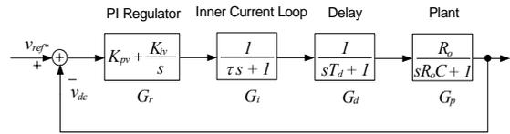
Figure 9. The plant and dc link voltage PI controller block diagram for the closed loop system with the delay element.
