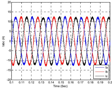
Figure 12. Simulated input current waveforms with observers resulting in 1.2% THD harmonic content.
