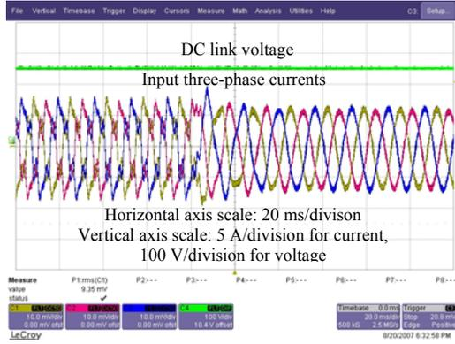
Figure 16. Experimental dc link voltage and input currents before and after compensation.
