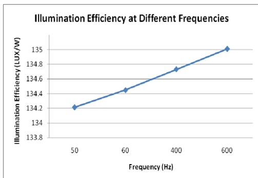
Fig.10 Illumination Efficiency of fluorescent lighting system.
