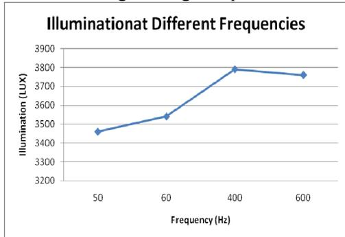
Fig.9 Illumination of fluorescent lighting system.
