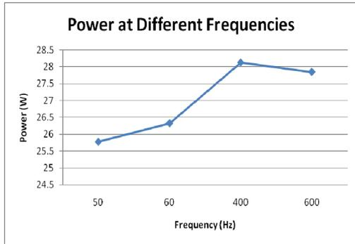
Fig.8 Input Power of fluorescent lighting system.
