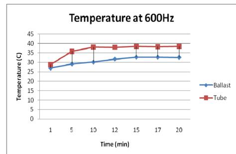
Fig.14. Temperature at 600Hz of fluorescent system.
