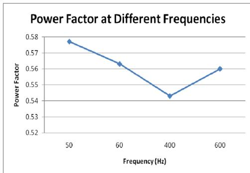
Fig.15 Power Factor of fluorescent lighting system.
