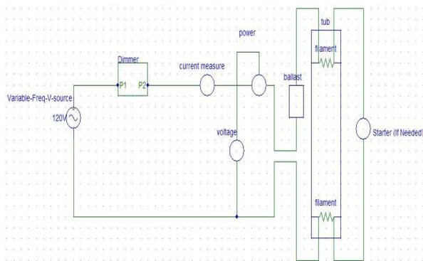
Fig. 2. Test Circuit for fluorescent lamp with magnetic ballast
