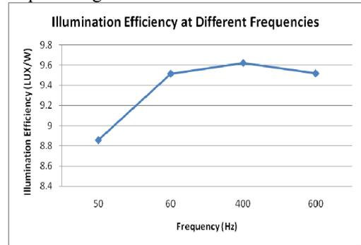
Fig. 6. Illumination Efficiency of incandescent Lamp.
