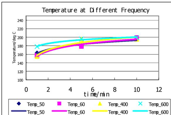
Fig. 4. Temperature of incandescent lamp.
