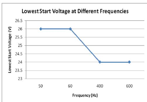
Fig.16 Lowest Start Voltage of fluorescent lighting
