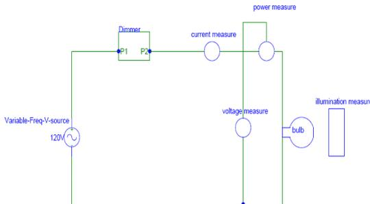
Fig. 1. Test Circuit for incandescent lamp
