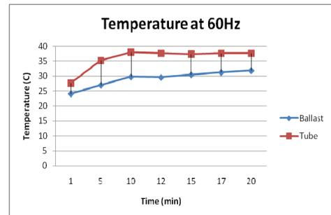
Fig.12. Temperature at 60Hz of fluorescent lighting system.
