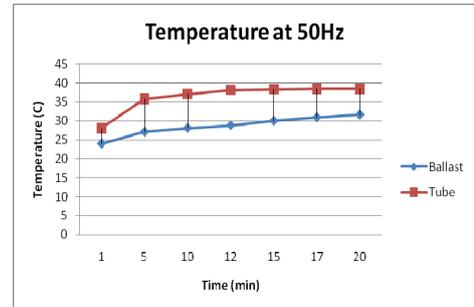
Fig.11. Temperature at 50Hz of Fluorescent lighting system.
