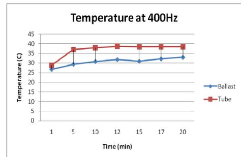
Fig.13 Temperature at 400Hz of fluorescent lighting system.
