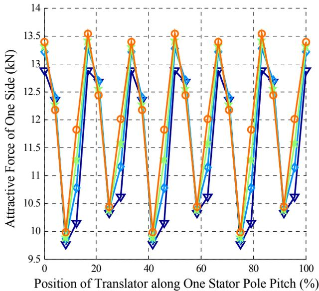
Figure 5. Attractive Force Variation of One Stator Side from FEA
