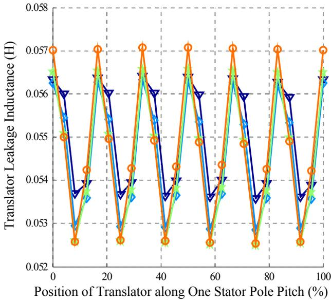
Figure 10. Translator Leakage Inductance Variation from FEA
