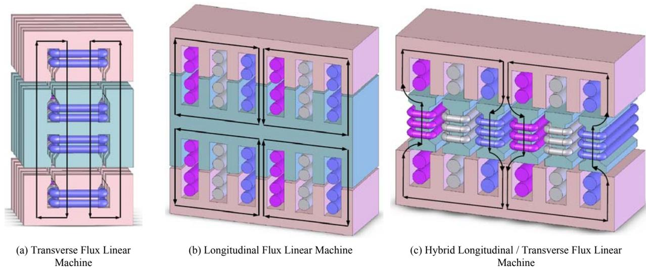
Figure 1. Flux Paths for One Pole Pair ( $q_s=1, q_r=1$ ) of Three Wound-Field Linear Machines
