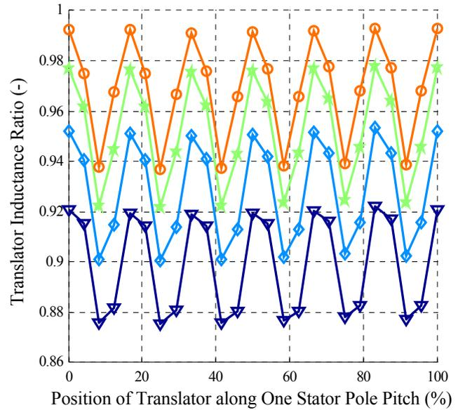
Figure 12. Variation of the Translator Magnetizing to Leakage Inductance Ratio from FEA
