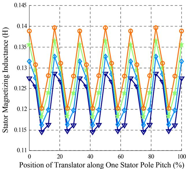
Figure 7. Stator Magnetizing Inductance Variation from FEA
