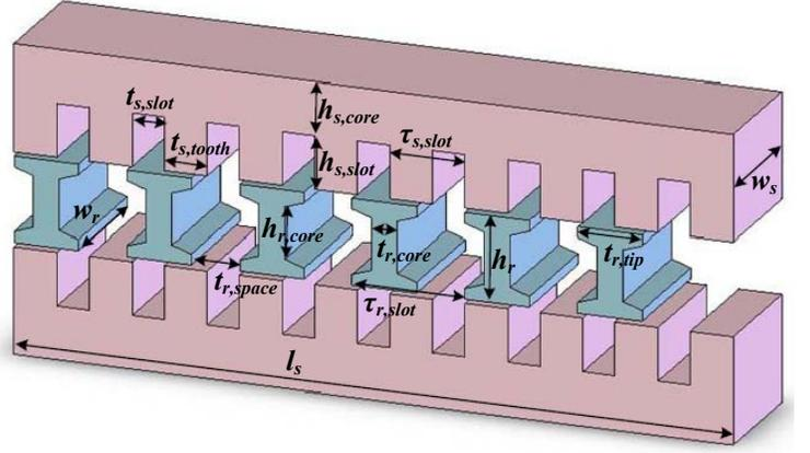
Figure 3. Linear Machine Physical Parameter Notation
