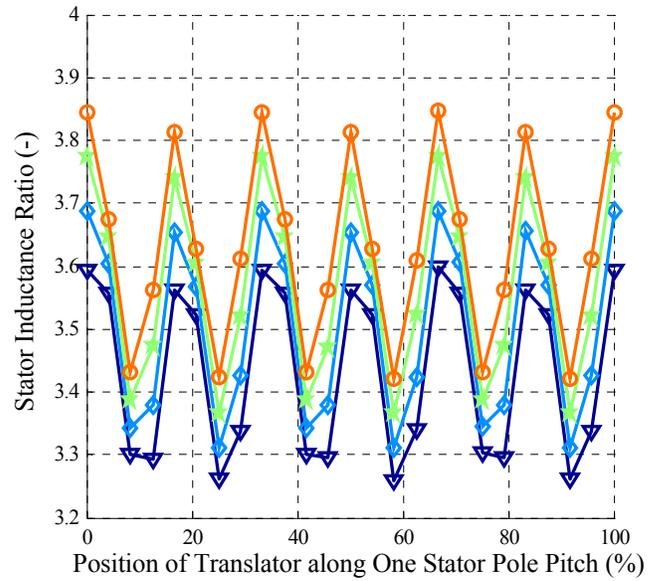
Figure 11. Variation of the Stator Magnetizing to Leakage Inductance Ratio from FEA
