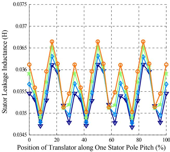
Figure 9. Stator Leakage Inductance Variation from FEA
