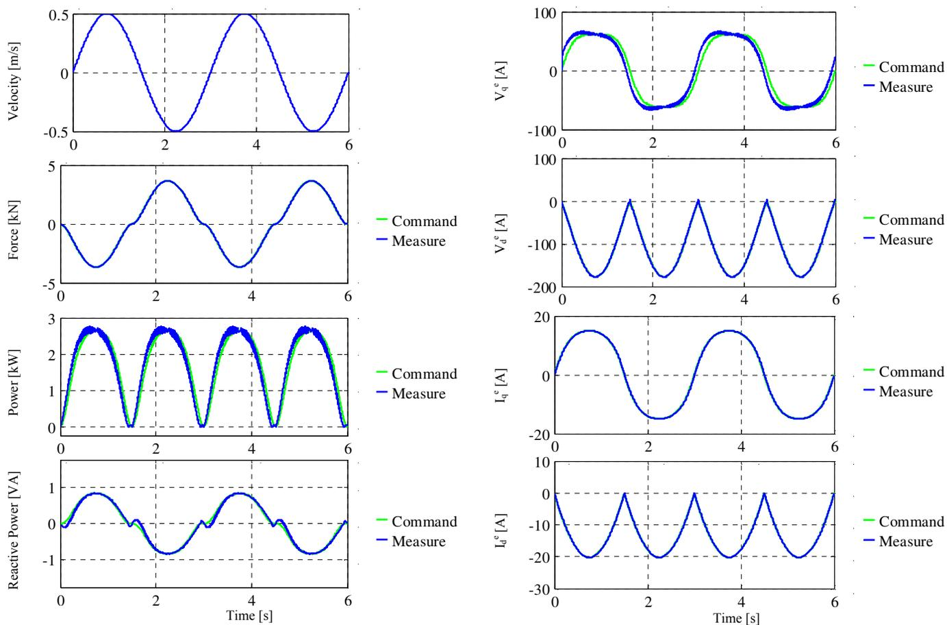
Figure 8. Waveforms obtained from computer simulation of the proposed system during a sinusoidal variation in the translator velocity
