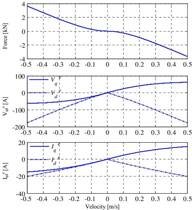
Figure 6. Constant V/Hz Maximum Power Command Trajectory
