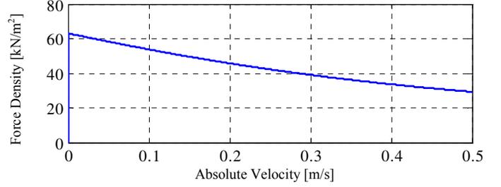
Figure 4. Steady State Maximum Generating Force Density vs. Velocity
