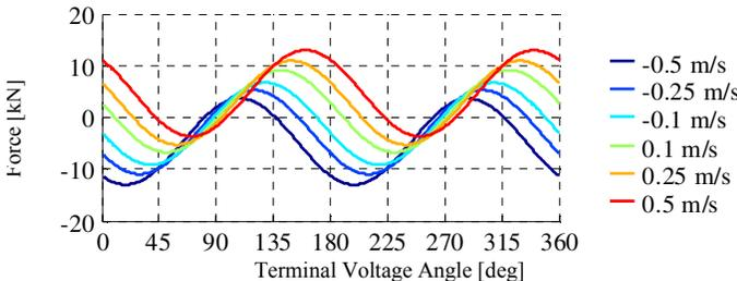
Figure 3. Steady State Force vs. Voltage Angle for Multiple Translator Velocities when Terminal Voltage Magnitude is held Constant
