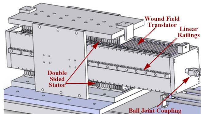
Figure 1. Hybrid Flux Linear Machine as developed in [1]
