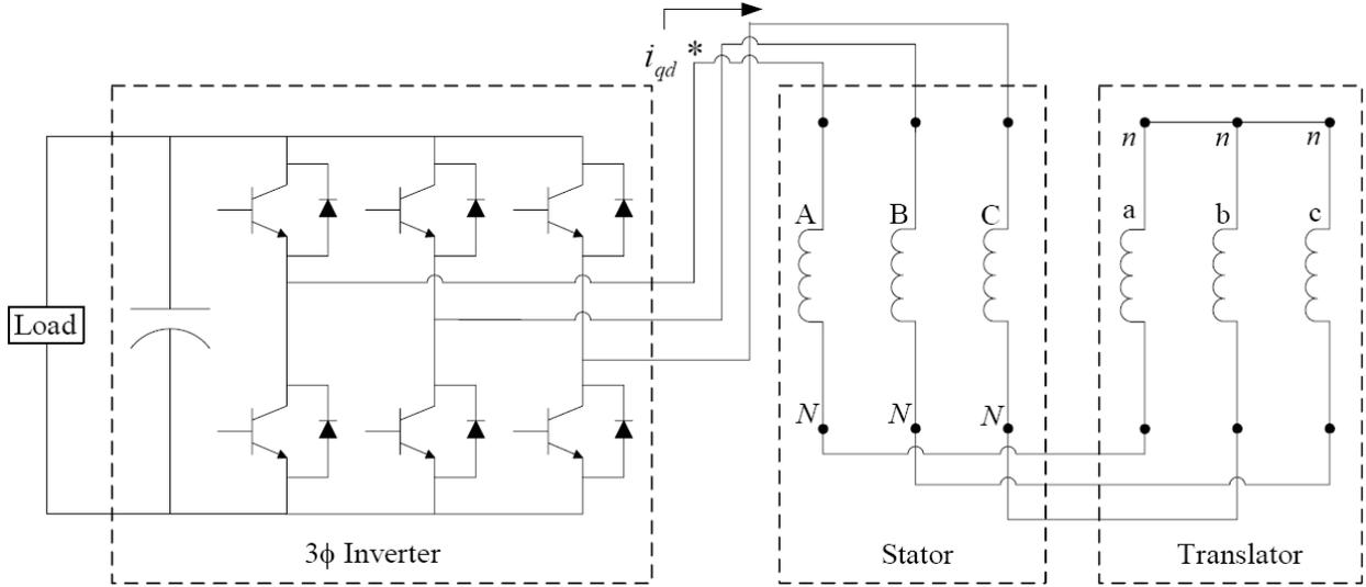
Figure 2. Power Circuit Interconnections for the Proposed Self-Synchronous Controller for the Doubly Fed Induction Generator
