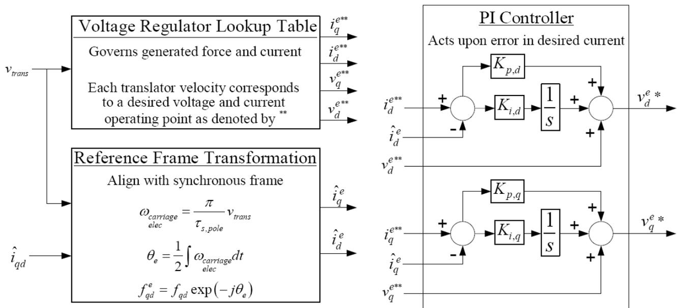
Figure 7. Self-Synchronous Maximum Power Controller Block Diagram
