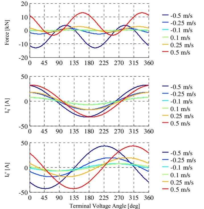
Figure 5. Steady State Force, Voltage, and Current vs. Voltage Angle for Multiple Translator Velocities when Terminal V/Hz is held Constant
