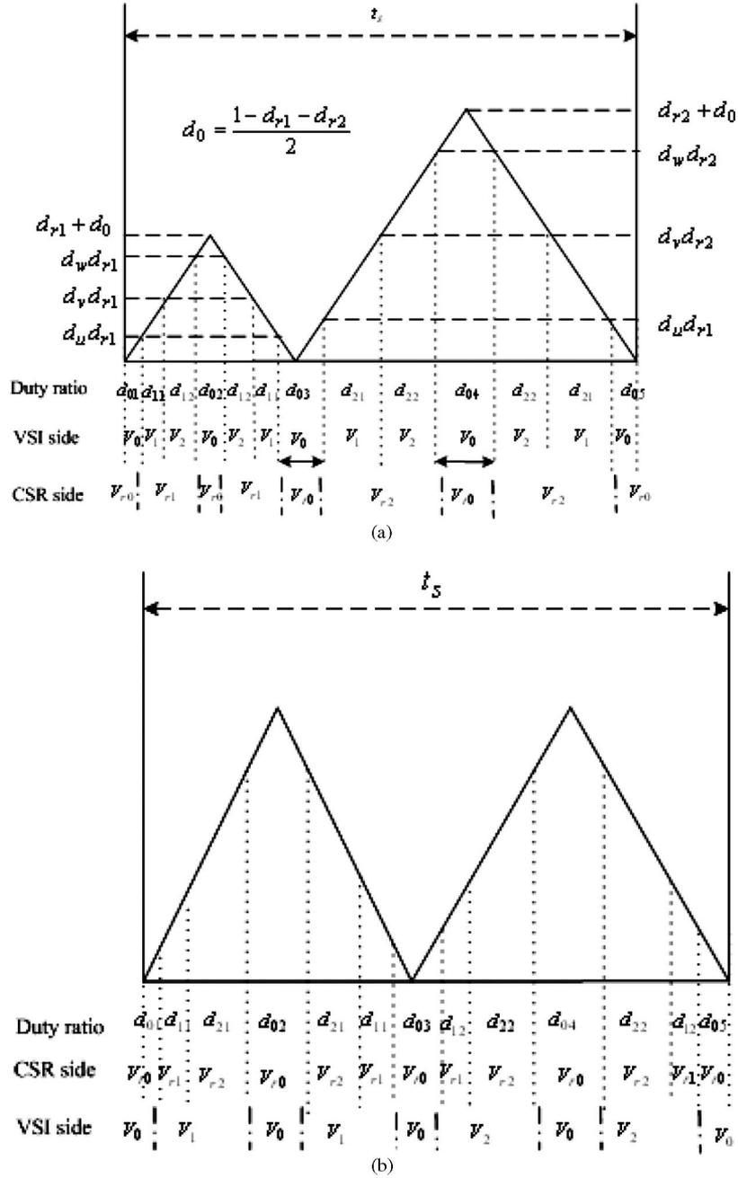
Fig. 4. ZCPWM and ZVPWM: (a) rectifier side ZCPWM and (b) inverter-side ZVPWM.
