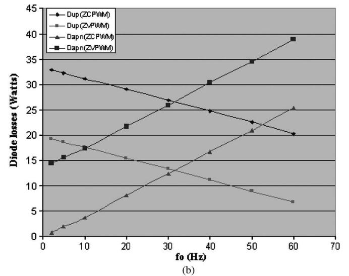
Fig. 5. Comparison of average power losses at different output frequency and rated output current (65 Arms) (a) IGBT losses comparison, (b) Diode losses comparison.
