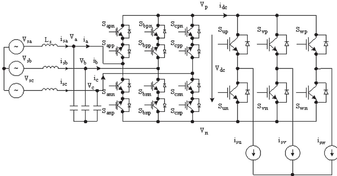
Fig. 1. 18-switch DBMC topology.
