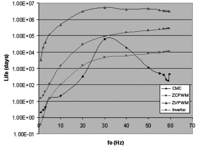
Fig. 8. Power cycling MTTF of the IGBT used in a DBMC, a CMC, and a dc/ac inverter at rated output current condition (65 Arms).
