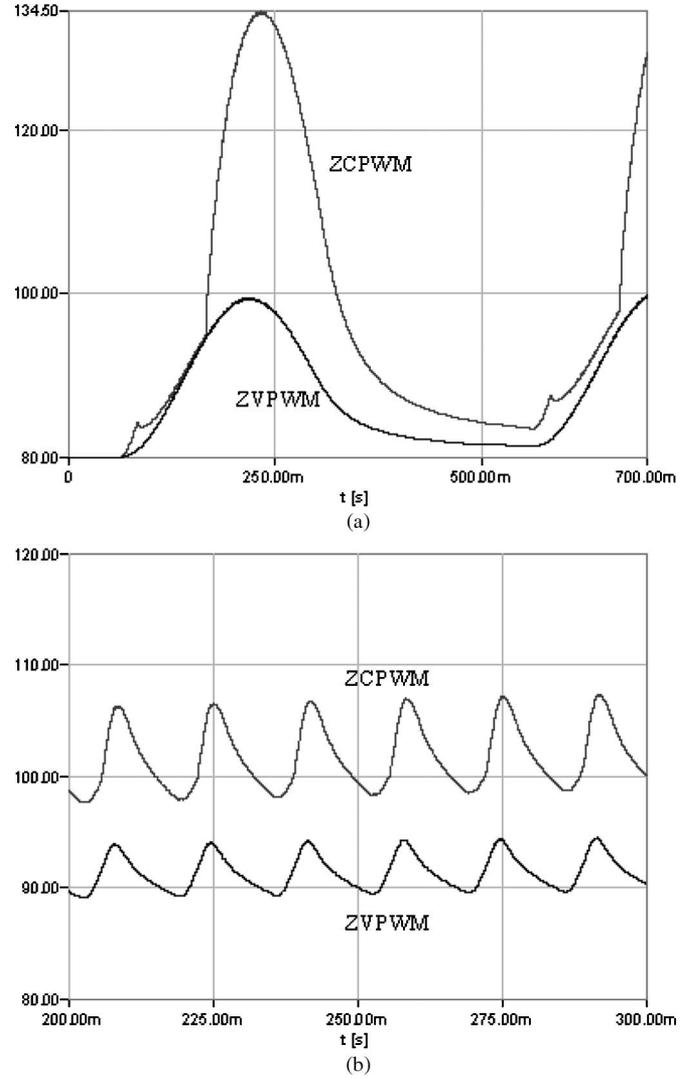
Fig. 7. Junction temperature profile of  $S_{up}$  at various output frequency under rated output current 65 Arms: (a) 2 Hz and (b) 60 Hz.
