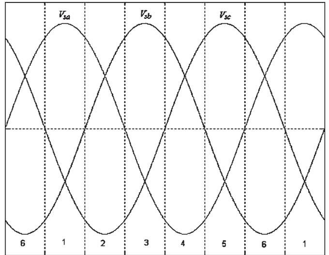
Fig. 2. Line-side intervals definition for the rectifier.
