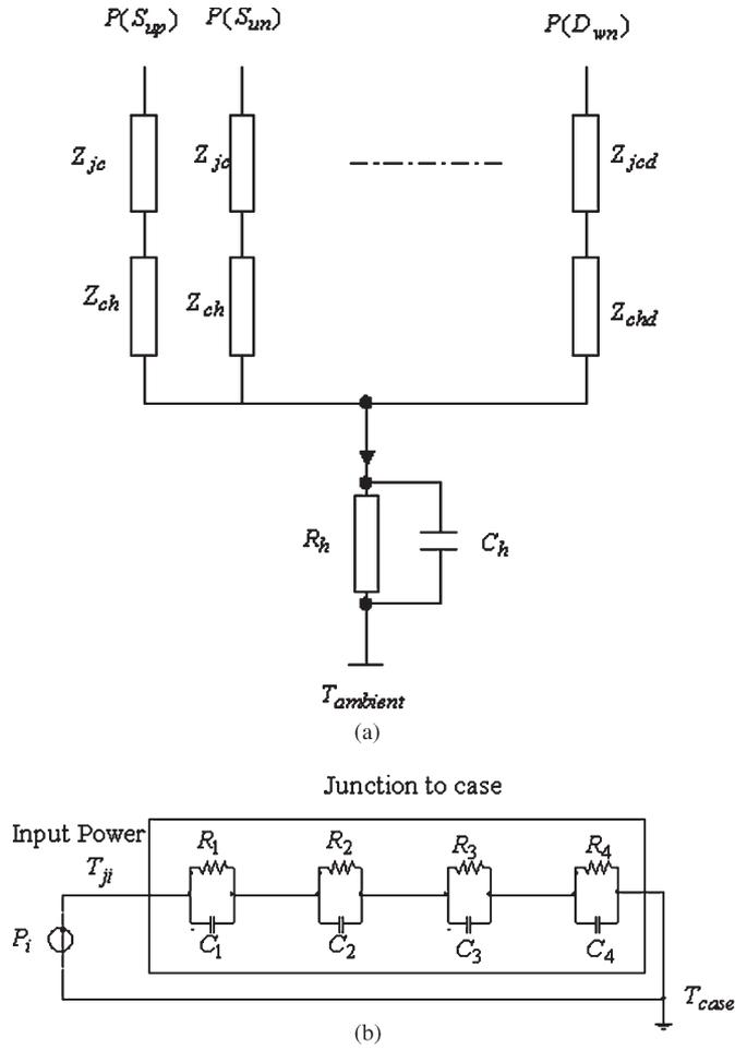
Fig. 6. Simplified thermal system of the DBMC: (a) overall thermal network model and (b) thermal impedance between the junction and case layer of one chip.
