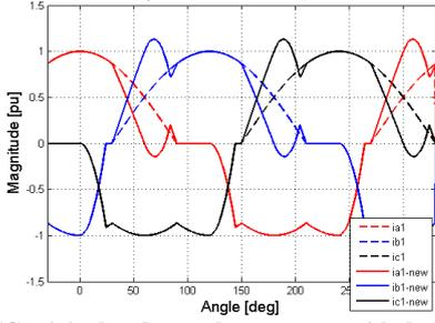
Fig. 4. HCC original and new phase current with desired (non-feasible) compensation
