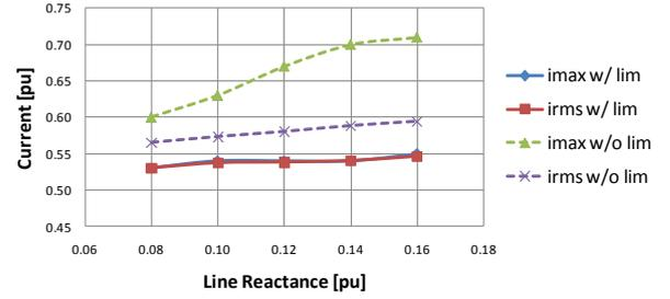
Fig. 20. Simulated current in HCC as a function of line reactance
