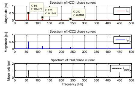
Fig. 17. Spectrum of DHCC current waveforms using coordinated volt-seconds modulation, with limiter
