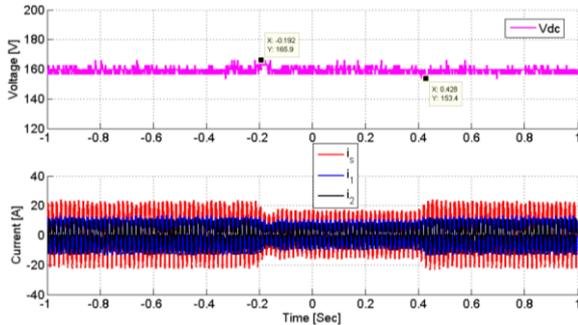
**Fig. 30. Experimental results: 25% load transients, DC-link voltage and DHCC currents, with peak current limiter**
