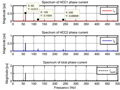
Fig. 13. Spectrums of DHCC current using formulated current compensation
