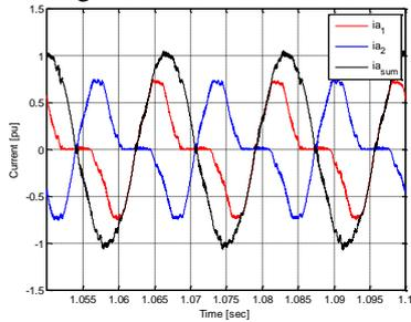
Fig. 14. DHCC current waveforms using coordinated volt-seconds modulation, without limiter
