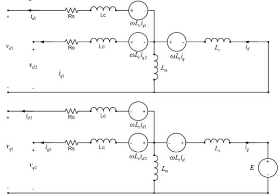
Fig. 7. D-axis (upper) and Q-axis (lower) equivalent circuits of DHCC rectifier system
