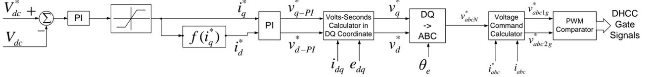
Fig. 9. Overall controller diagram of coordinated volt-second modulation
