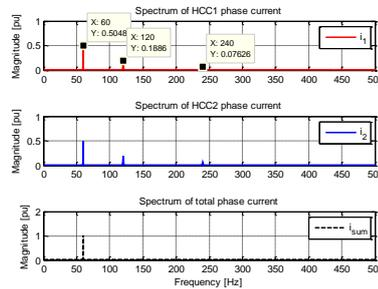
Fig. 11. Spectrums of DHCC current waveforms using current command cross-coupling
