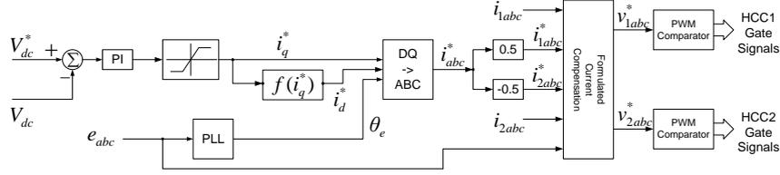
Fig. 8. Overall controller diagram of formulated current compensation
