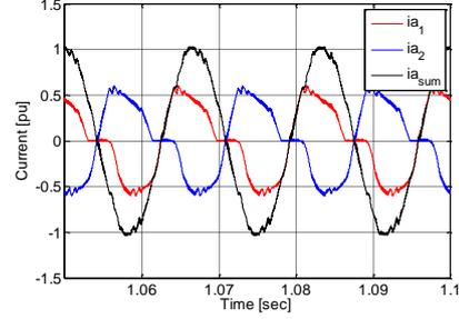
Fig. 16. DHCC current waveforms using coordinated volt-seconds modulation, with limiter
