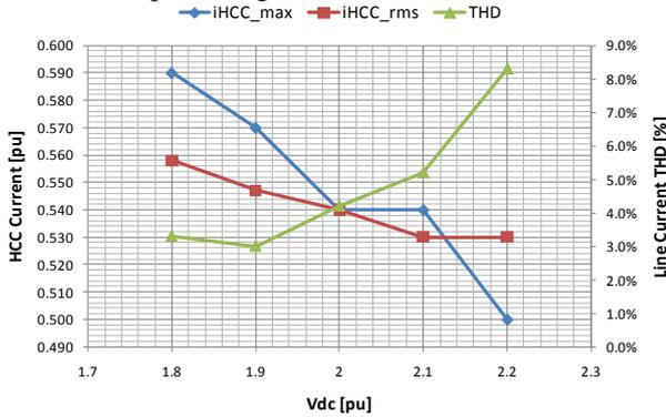
Fig. 24. Current rating and THD as functions of DC-link voltage
