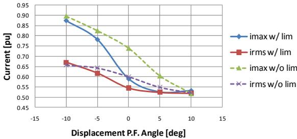
**Fig. 29. Experimental results: maximum and RMS currents in each HCC with and without peak current limiter**
