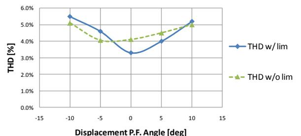
Fig. 23. Current THD as a function of power factor angle
