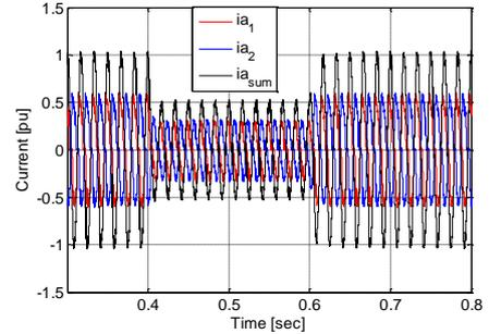
Fig. 18. DHCC phase currents during load transient
