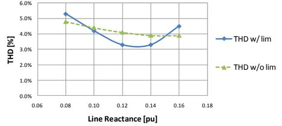
Fig. 21. Simulated current THD as a function of line reactance
