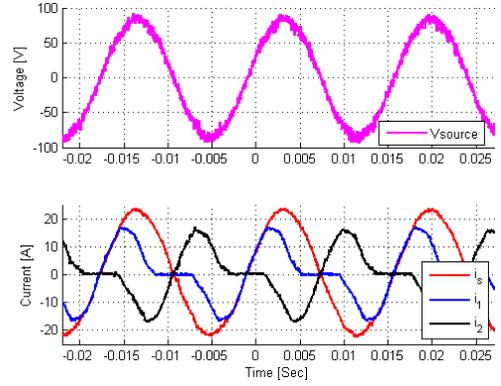
Fig. 25. Experimental results at unity power factor without peak current limiter in each HCC; upper: source voltage; lower: total current and currents in both HCCs
