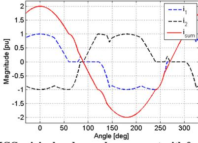
Fig. 5. HCC original and new phase current with feasible but compromised compensation
