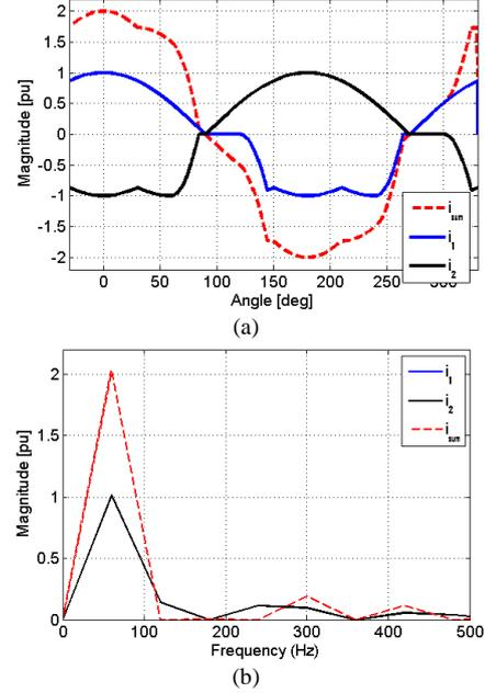
Fig. 3. DHCC phase current without active compensation, (a) waveforms, and (b) spectrums
