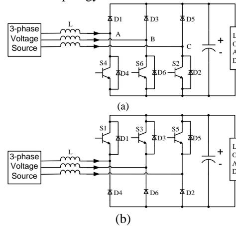
Fig. 1. HCC configurations: CE (a) and CC (b) [1]
