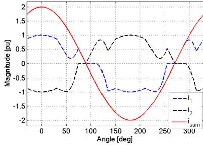
Fig. 6. HCC original and new phase current with compensation at 10 degrees lagging power factor
