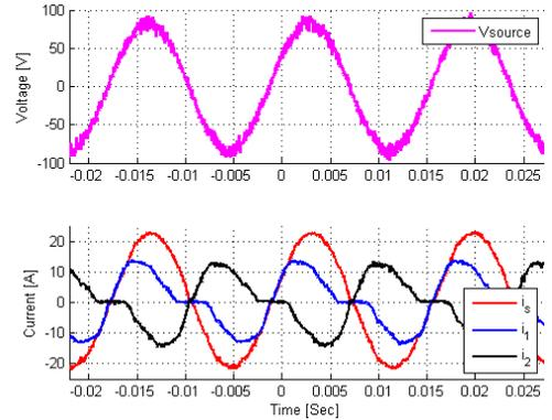
Fig. 27. Experimental results at 5 degrees lagging power factor without peak current limiter in each HCC; upper: source voltage; lower: total current and currents in both HCCs
