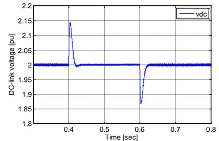
Fig. 19. DHCC DC-link voltage during load transient
