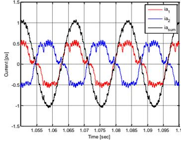
Fig. 12. DHCC current waveforms using formulated current compensation
