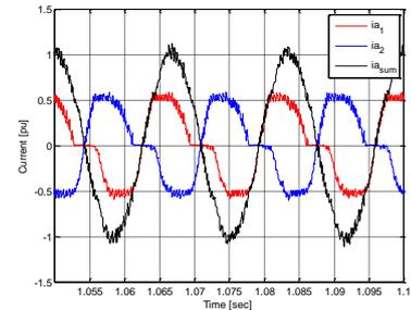
Fig. 10. DHCC current waveforms using current command cross-coupling
