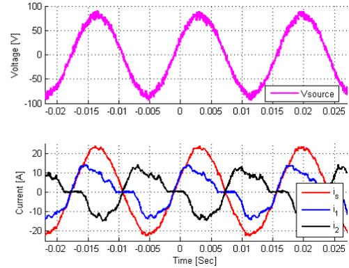
Fig. 26. Experimental results at unity power factor with peak current limiter in each HCC; upper: source voltage; lower: total current and currents in both HCCs
