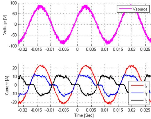
**Fig. 28. Experimental results at 5 degrees lagging power factor with peak current limiter in each HCC; upper: source voltage; lower: total current and currents in both HCCs**
