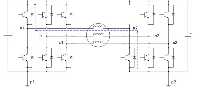
Fig. 13. Illustration of an open-switch fault
