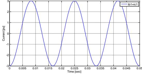
Fig. 11. Zero-sequence current in 2-phase mode
