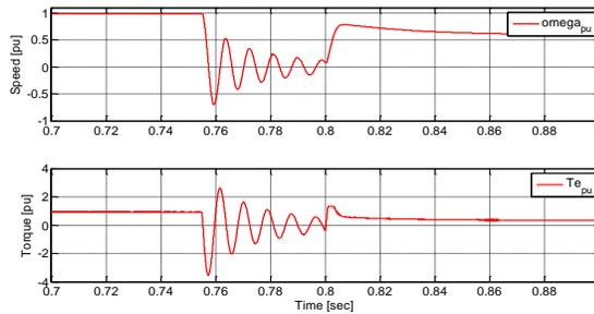
Fig. 6. Rotor speed and developed torque
