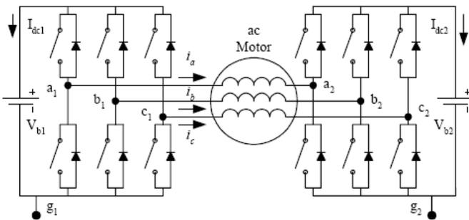
Fig. 1. Double-output AC machine drive
