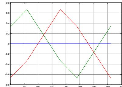
Fig. 9. Phase currents  $i_b$  and  $i_c$  after subtracting the zero component
