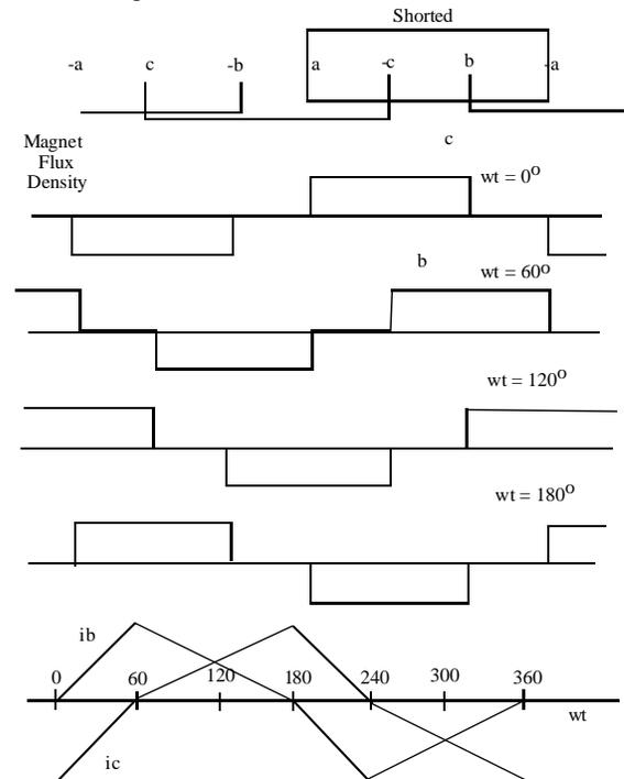
Fig. 8. Top trace: full pitch winding layout; next four traces: four positions of the magnet flux with respect to the stator windings; bottom trace: phase *b* and *c* current needed to reduce the magnet flux linking phase *a*
