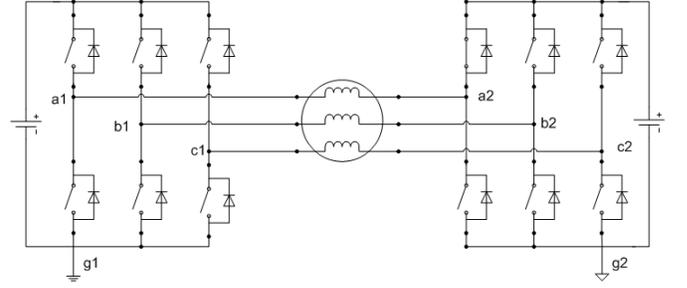
Fig. 2. Short-circuit fault in  $a2$  upper switch
