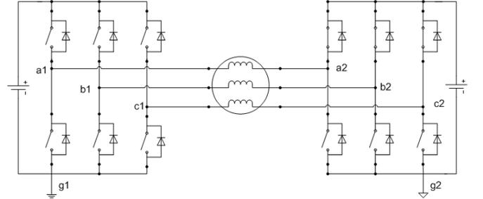
Fig. 3. Artificial neutral in case of shorted-switch fault
