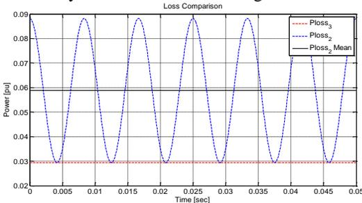
Fig. 12. Stator loss comparison, 2-phase mode v.s. 3-phase mode
