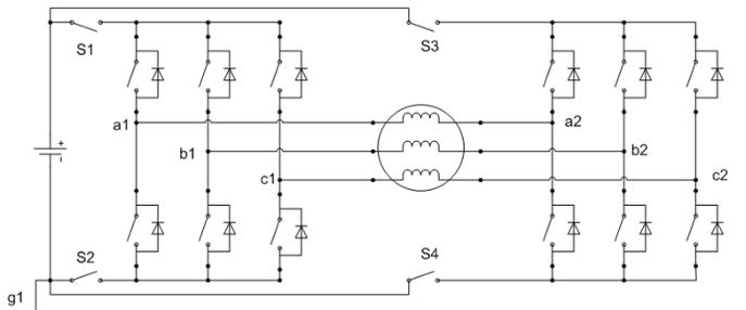
Fig. 4. Double-output inverter with contactors on the DC link
