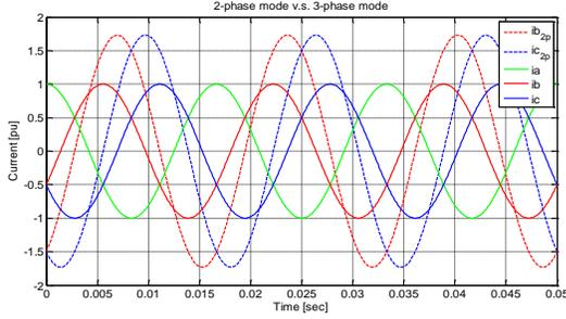
Fig. 10. Phase currents in 2-phase and 3-phase mode
