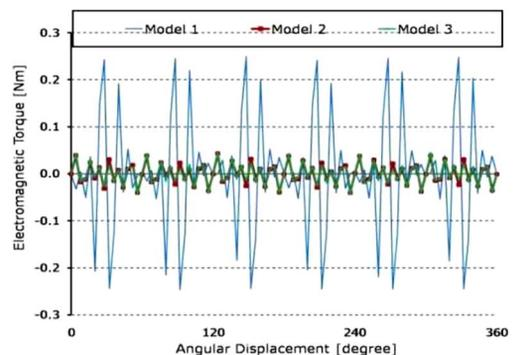
Fig. 6. Cogging torque of SPM motor models.
