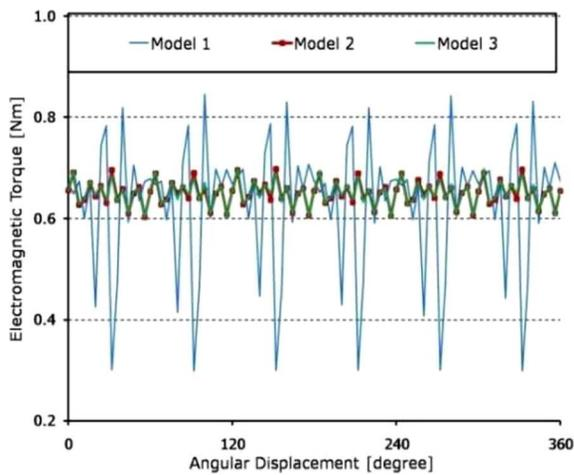
Fig. 8. Electromagnetic torque when sinusoidal current waveform excitation is supplied.
