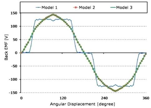
Fig. 5. Back EMF waveform of phase A of SPM motor models.
