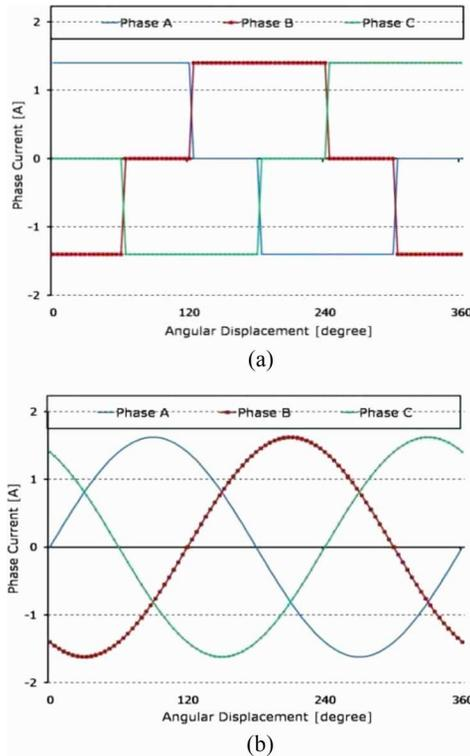
Fig. 4. Stator current excitation source. (a) Square current. (b) Sinusoidal current.
