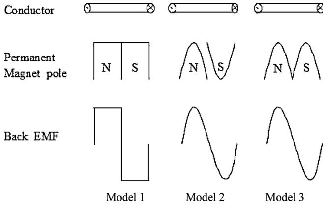
Fig. 2. Schematic diagram of SPM motor models and their back EMF generation.
