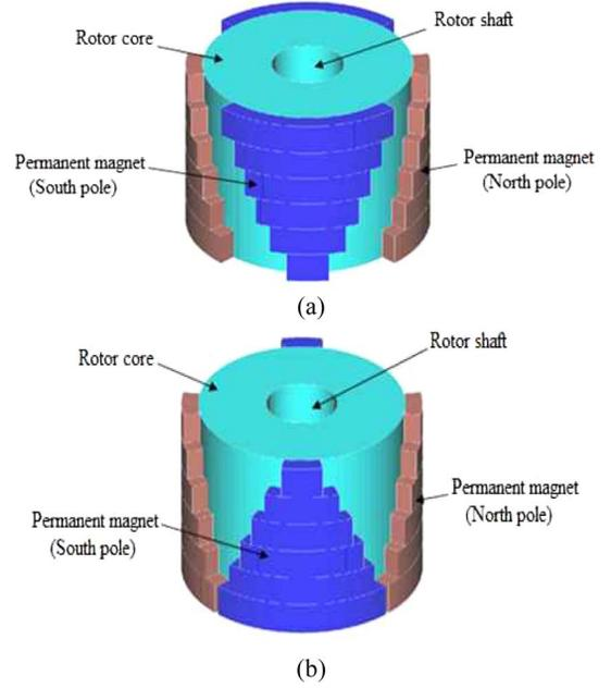
Fig. 3. PM structure of the proposed SPM motor models. (a) Model 2. (b) Model 3.
