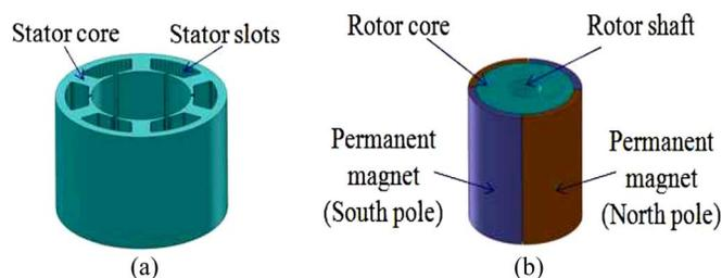
Fig. 1. Conventional SPM motor structure. (a) Stator. (b) Rotor.
