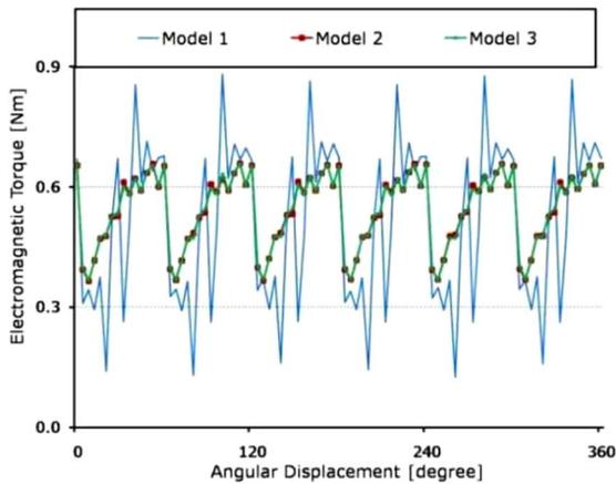
Fig. 7. Electromagnetic torque when square current waveform excitation is supplied.
