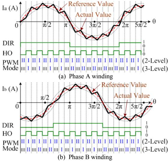
Fig. 6. PWM scheme for three-level modulation
