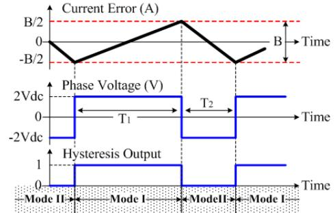
Fig. 4. Hysteresis operation with two-level modulation
