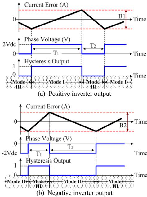
Fig. 5. Hysteresis operation with three-level modulations for positive inverter output
