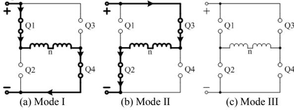
Fig. 3. Three operation modes of one phase inverter
