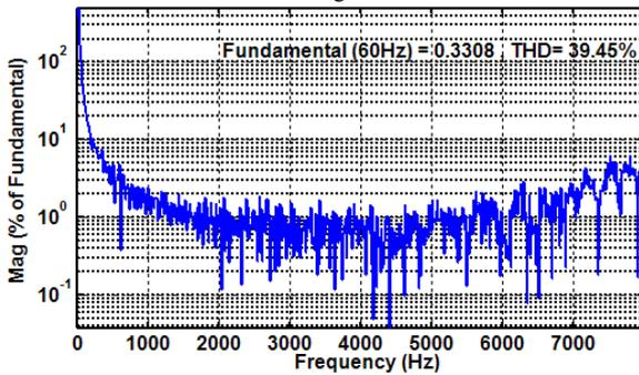
(b) Two-level hysteresis controller with variable band for eight-switch inverter of figure 2
