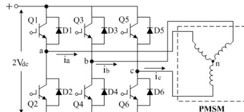
Fig. 1. Traditional six-switch inverter configuration for three-phase PMSM drive under two-level modulation
