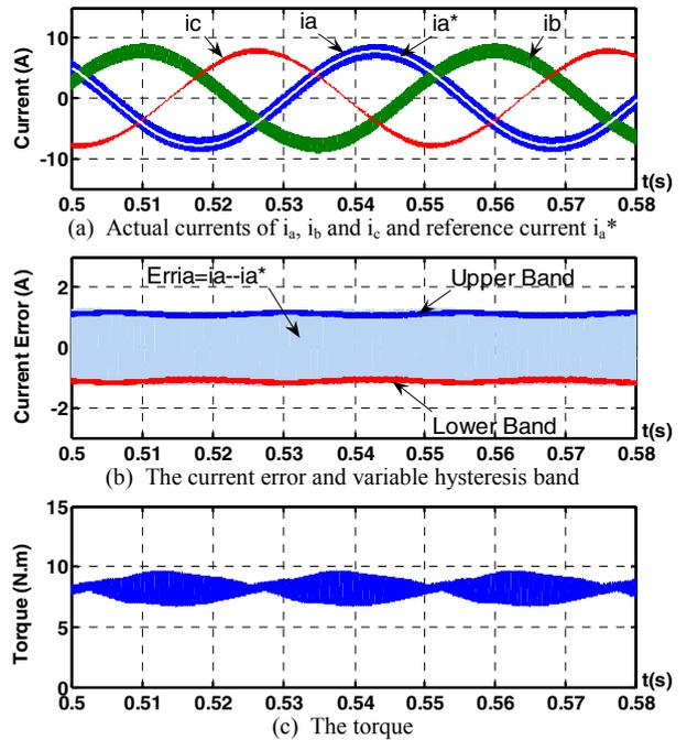
Fig. 8. Two-level hysteresis controller with variable band for three-phase PMSM drives
