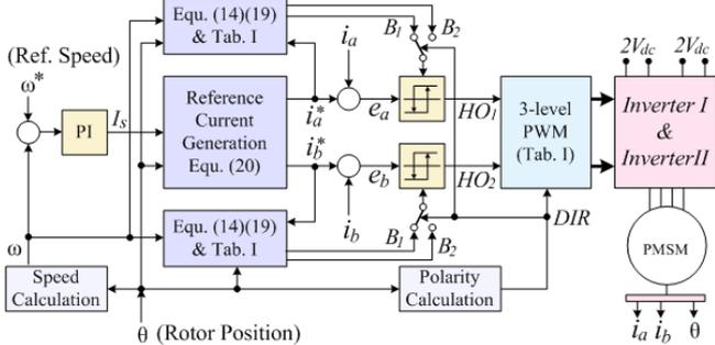
Fig. 7. The configuration of the proposed three-level hysteresis modulation for three-phase PMSM drives
