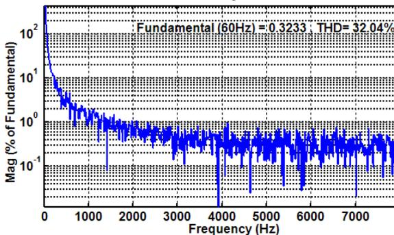
(c) Three-level hysteresis controller with variable band for eight-switch inverter of figure 3
