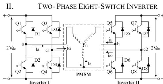
Fig. 2. Proposed eight-switch inverter configuration for three-phase PMSM drive under three-level modulation
