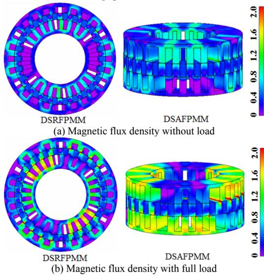
Fig. 5. Magnetic flux density distribution.
