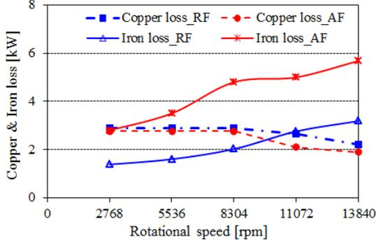
Fig. 12. Copper loss and iron loss over the constant power region.
