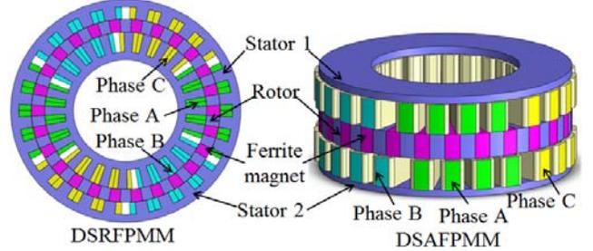
Fig. 3. Topologies of DSRFPMM and DSAFPMM.
