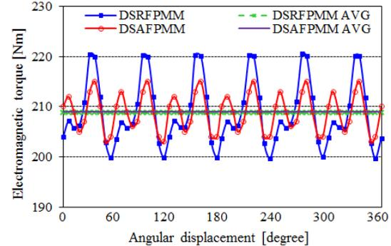
Fig. 9. Electromagnetic torque with respect to rotational angle.
