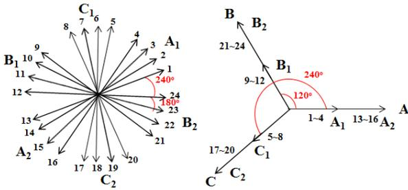
Fig. 2. Winding configuration and resultant EMF vector.
