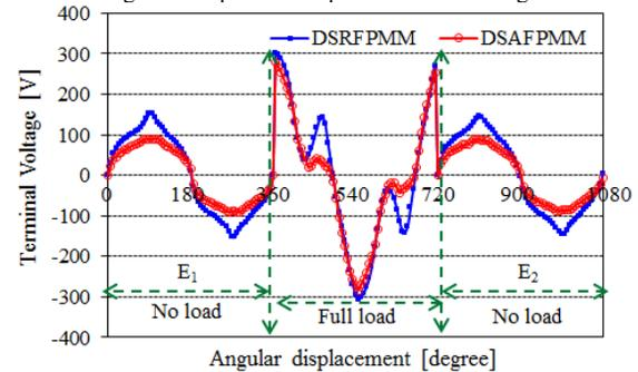
Fig. 10. Terminal voltage with no load and full load.
