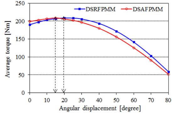
Fig. 8. Average torque with respect to current phase angle.
