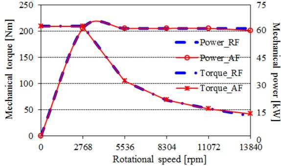
Fig. 11. Constant torque and constant power region with FW control.
