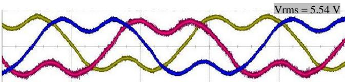
Fig. 14. Back EMF of the machine during mode-1 operation
