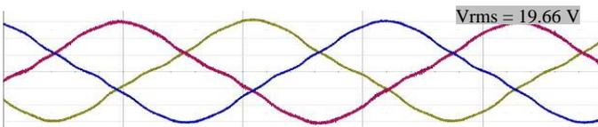
Fig. 13. Back EMF of the machine during mode-1 operation
