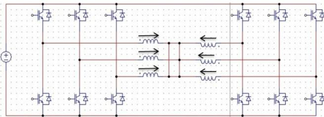
Fig. 2. Winding configuration before switching.
