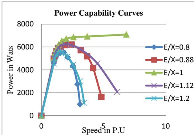
Fig. 8. Power capability curves of the machines with different E/X
