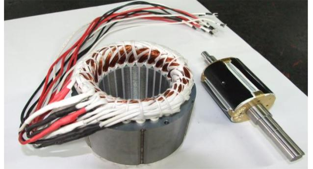
Fig. 11. Rotor and Stator of the machine being used for experiment
