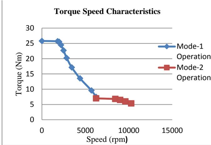
Fig. 9. Speed Torque characteristic curve.
