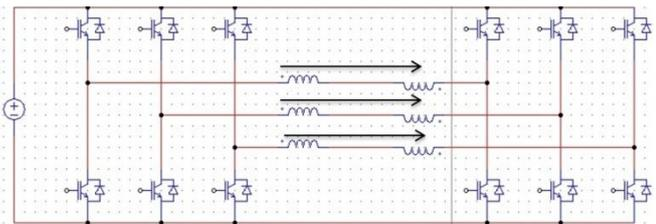
Fig. 3. Winding configuration after winding switching.
