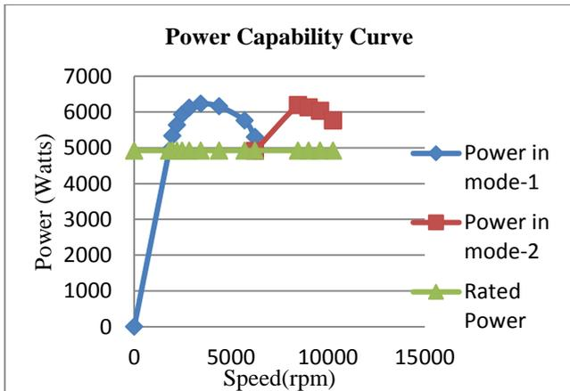
Fig. 10. Power capability curve of the machine for mode-1 and mode-2
