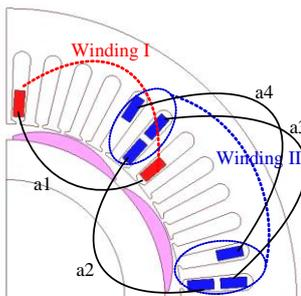
Fig. 7. Two layer lap winding of stator phase A
