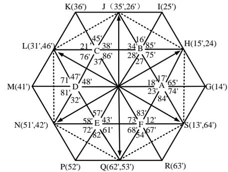
Fig. 3. The space vector and combinations of dual 2-level inverter
