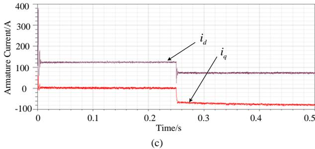
Fig. 9. Middle speed region to FW region. (a) Speed.(b) Torque.(c) Armature current.
