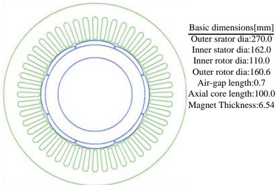
Fig. 6. Basic dimension of the drive motor
