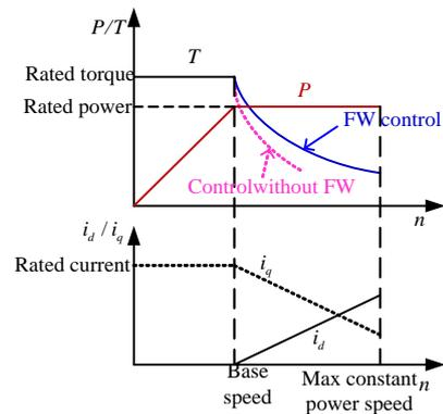
Fig. 1. Traditional operating strategy for control of a PMSM
