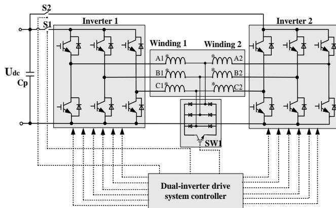
Fig. 2. The dual inverter-fed drive system
