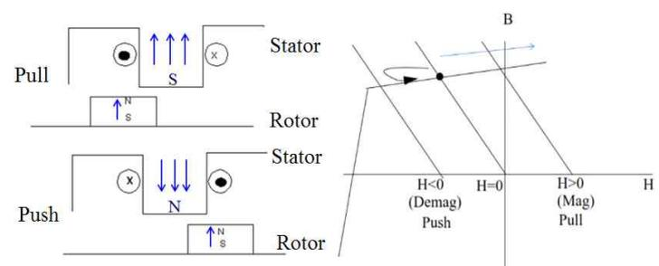
Fig. 1 Basic operation principle of only pull process
