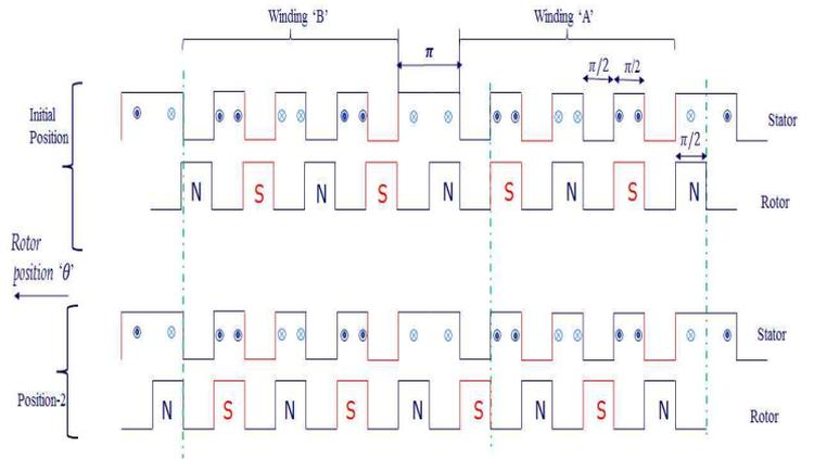
Fig.4. Pull process and rotor position
