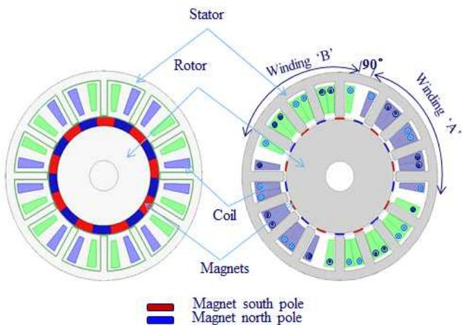
Fig.3. Two phase brushless DC machine (a) conventional machine, 12slot/18pole (b) proposed machine, 16slots/18pole
