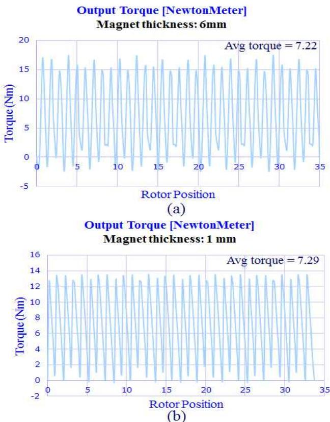
Fig.6. Output Torque (a) for conventional model (b) for proposed model
