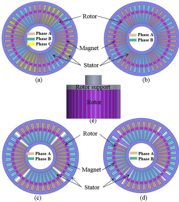
Fig. 1. Machine topologies. (a) Conventional three-phase PMSM (Model 1). (b) Conventional two-phase PMSM (Model 2). (c) Proposed two-phase PMSM-slot (Model 3). (d) Proposed two-phase PMSM-teeth (Model 4). (e) Rotor-PM configuration.
