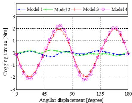
Fig. 7. Comparison of cogging torques.
