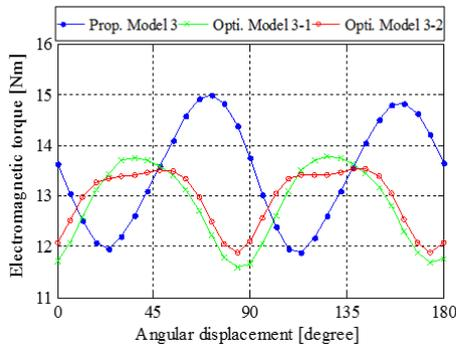
Fig. 12. Electromagnetic torques of the proposed and optimized model 3.
