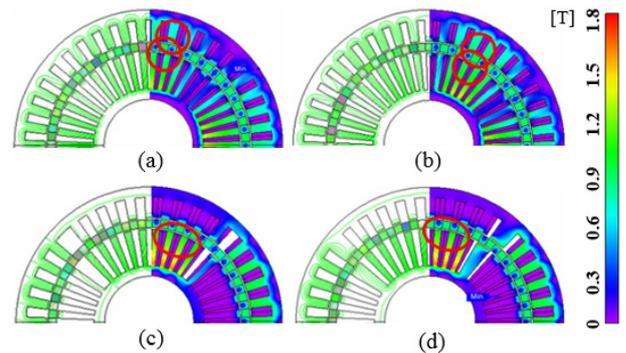
Fig. 3. Magnetic flux density distribution. (a) Conventional model 1. (b) Conventional model 2. (c) Proposed model 3. (d) Proposed model 4.
