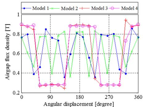
Fig. 4. Comparison of airgap flux density.
