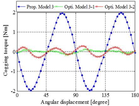
Fig. 11. Cogging torques of the proposed and optimized model 3.
