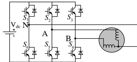
Fig. 1. Schematic diagram of an inverter.
