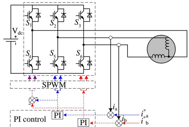
Fig.3. Block diagram of conventional 2 PI control.
