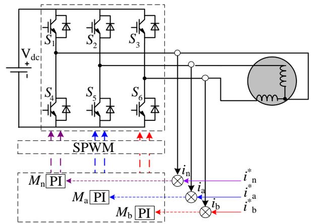
Fig. 2. Block diagram of 3 PI control.
