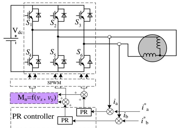
Fig. 4. Block diagram of proposed control.
