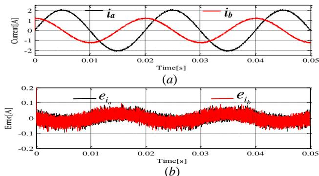
Fig. 6. Output currents and errors of method I, (a), output currents, (b), errors.
