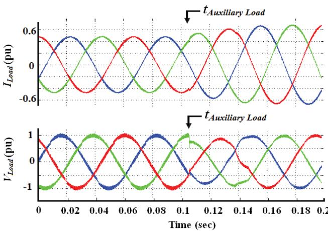
Figure 13: Transient behaviour of line-interactive UPS system during switching-in of an auxiliary load at 210° of phase A, while feeding a main load with the proposed control scheme.
