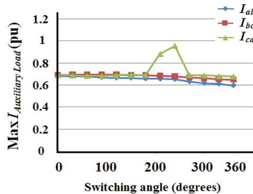
Figure 16: Effect on the magnitude of  $I_{Auxiliary Load}$  for the line-interactive UPS system during switching-in of auxiliary load while feeding a main load with the proposed control scheme.
