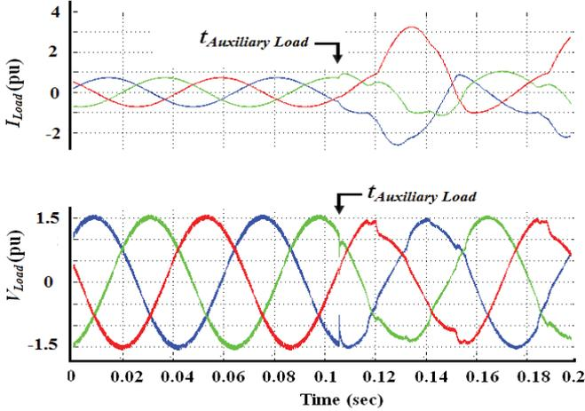
Figure 6: Transient behaviour of line-interactive UPS system during switching-in of an auxiliary load at  $210^\circ$  of phase A, while feeding a main load without the proposed control scheme.
