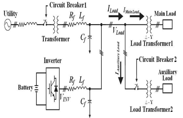
Figure 1: One-line diagram of the proposed line-interactive UPS system with the main and auxiliary loads.
