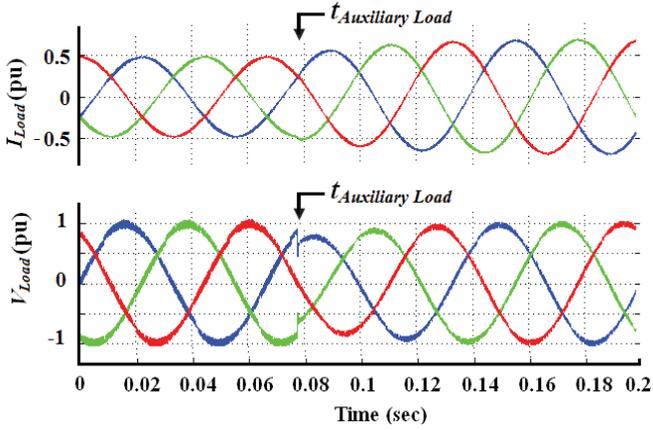
Figure 11: Transient behaviour of line-interactive UPS system during switching-in of an auxiliary load at 60° of phase A, while feeding a main load with the proposed control scheme.
