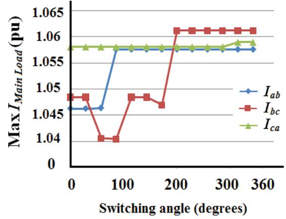
Figure 8: Effect on the magnitude of  $I_{Main Load}$  for the line-interactive UPS system during switching-in of an auxiliary load while feeding a main load without the proposed control scheme.
