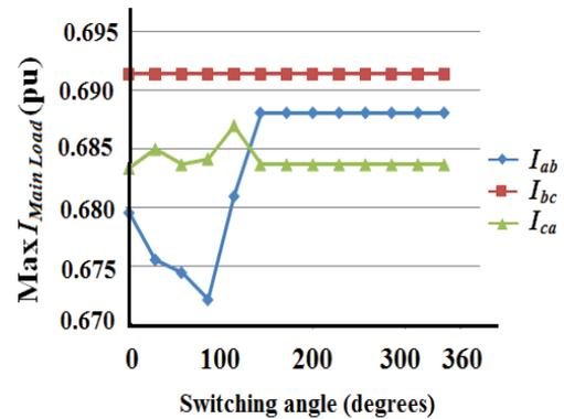
Figure 15: Effect on the magnitude of  $I_{Main Load}$  for the line-interactive UPS system during switching-in of auxiliary load while feeding a main load with the proposed control scheme.
