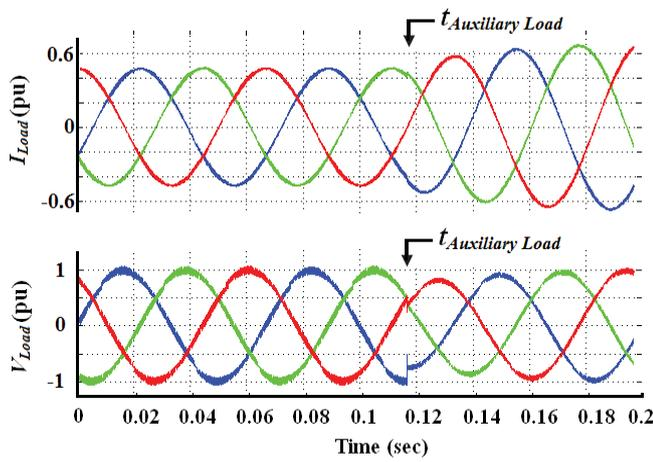
Figure 12: Transient behaviour of line-interactive UPS system during switching-in of an auxiliary load at 270° of phase A, while feeding a main load with the proposed control scheme.
