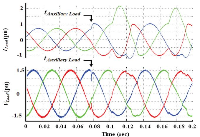
Figure 4: Transient behaviour of line-interactive UPS system during switching-in of an auxiliary load at 60° of phase A, while feeding a main load without the proposed control scheme.
