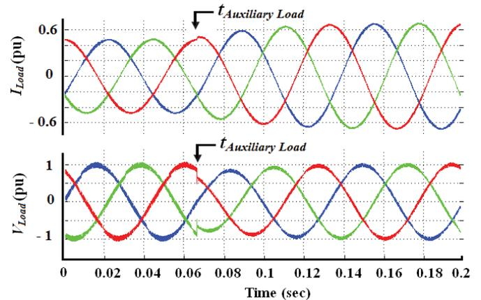
Figure 10: Transient behaviour of line-interactive UPS system during switching-in of an auxiliary load at  $0^\circ$  of phase A, while feeding a main load with the proposed control scheme.
