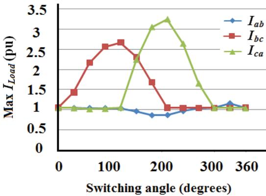
Figure 7: Effect on the magnitude of  $I_{Load}$  for the line-interactive UPS system during switching-in of an auxiliary load while feeding a main load without the proposed control scheme.
