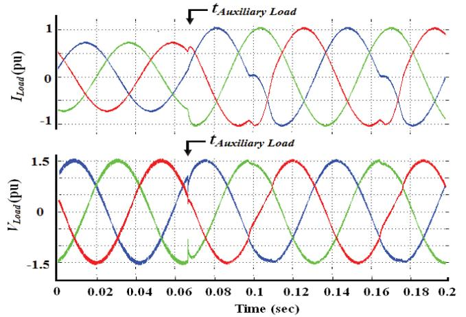
Figure 3: Transient behaviour of line-interactive UPS system during switching-in of an auxiliary load at 0° of phase A, while feeding a main load without the proposed control scheme.
