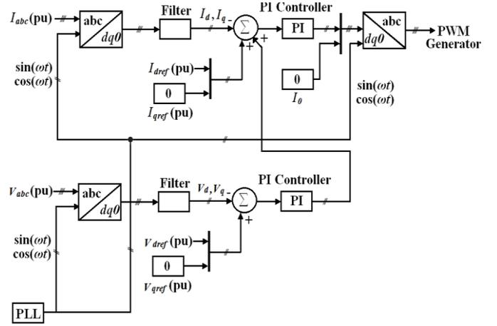
Figure 2: Proposed control scheme for the inverter in  $dq0$  frame of reference
