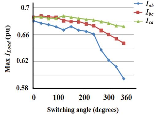
Figure 14: Effect on the magnitude of  $I_{Load}$  for the line-interactive UPS system during switching-in of auxiliary load while feeding a main load with the proposed control scheme.
