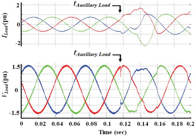
Figure 5: Transient behaviour of line-interactive UPS system during switching-in of an auxiliary load at  $270^\circ$  of phase A, while feeding a main load without the proposed control scheme.
