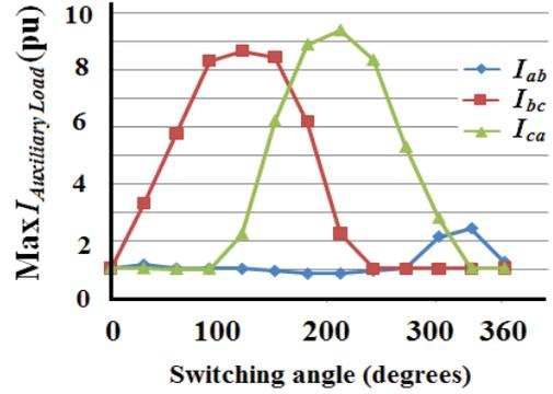
Figure 9: Effect on the magnitude of  $I_{Auxiliary Load}$  for the line-interactive UPS system during switching-in of an auxiliary load while feeding a main load without the proposed control scheme.
