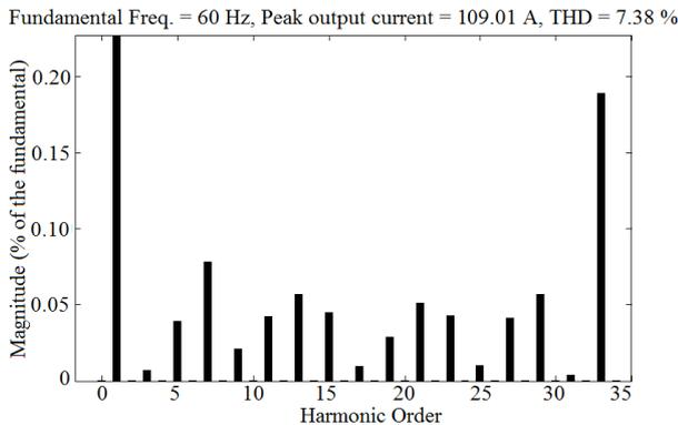
Fig. 9. THD of the output current of the utilizing SVPWM
