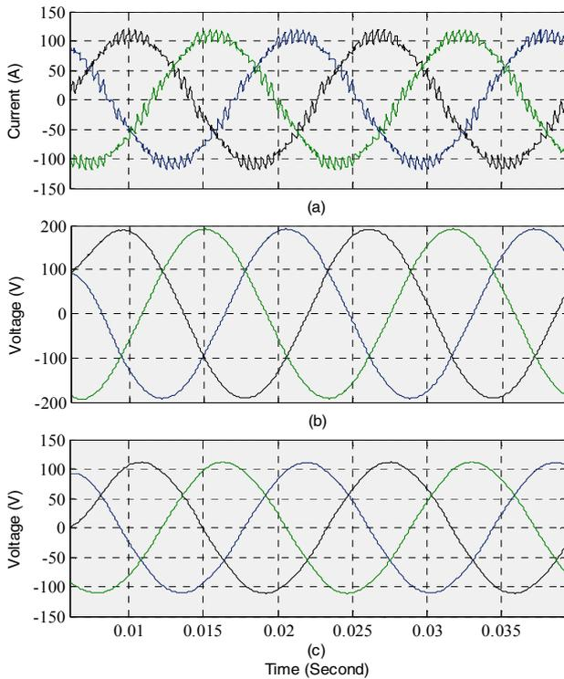
Fig. 8. Simulation result of the TTVSI topology utilizing SVPWM technique, a) three phase output currents; (b) output line voltages; (c) output phase voltages
