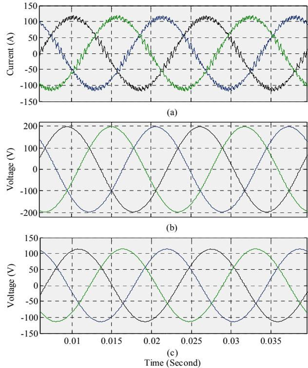
Fig. 10. Simulation result of the CVSI topology using the SVPWM technique, a) three phase output currents; (b) output line voltages; (c) output phase voltages
