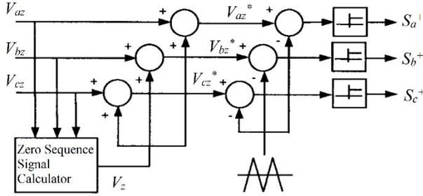
Fig. 3. The signal block diagram of the triangle intersection technique-based PWM employing the zero-sequence injection principle.
