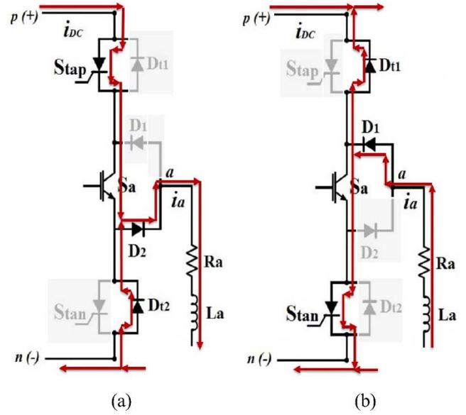
Fig. 2. Basic operation and the commutation technique for phase “a”: (a) positive, and (b) negative current flow.
