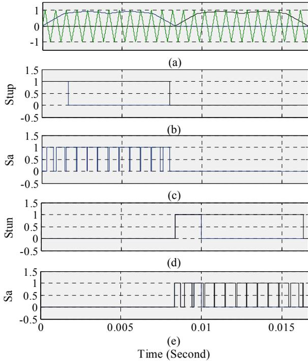
Fig. 5. PWM generation and switching pulses (a) SVPWM pulse generation method; (b) and (d) thyristor firing pulses and their conduction periods; (c), and (e) transistors switching pulses.
