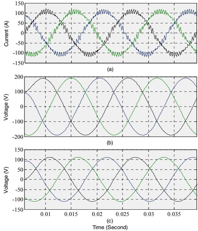
Fig. 6. Simulation result of the TTVSI topology utilizing TH-SVPWM technique, (a) three phase output currents; (b) output line voltages; (c) output phase voltages
