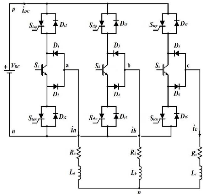
Fig. 1. Schematic of the three transistor VSI topology
