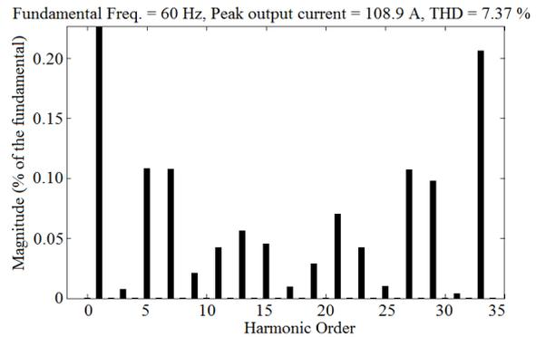
Fig. 7. THD of the output current utilizing TH-SVPWM
