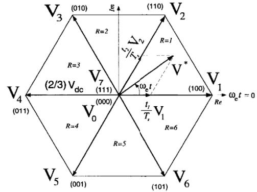
Fig. 4. The space vector diagram and its different sectors.
