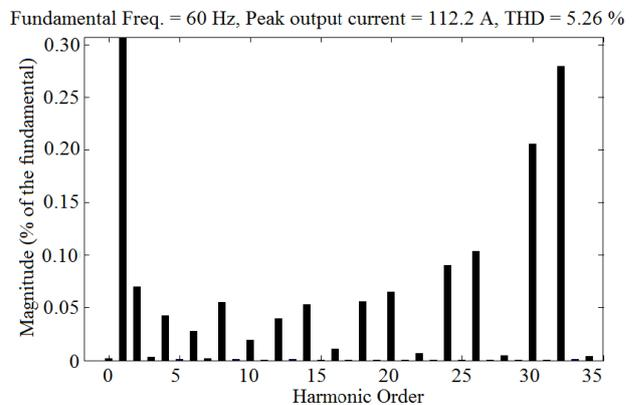
Fig. 11. THD of the output current of the conventional VSI using SVPWM method
