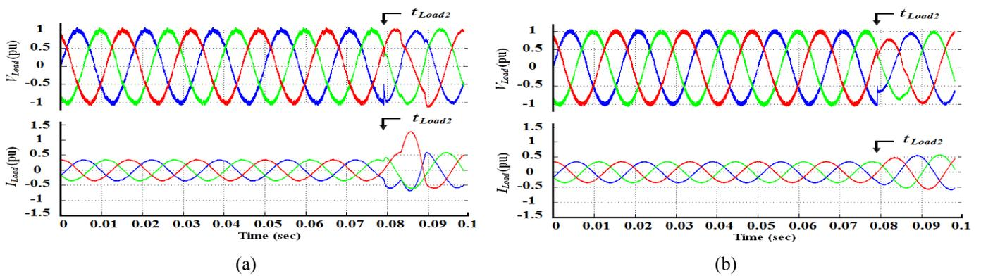
Fig. 8. Transient performance of the on-line UPS system when load transformer2 is switched in at an angle of 270 deg. of phase A. (a)  $I_{Load}$  and  $V_{Load}$  for the conventional UPS system, (b)  $I_{Load}$  and  $V_{Load}$  for the proposed UPS system.
