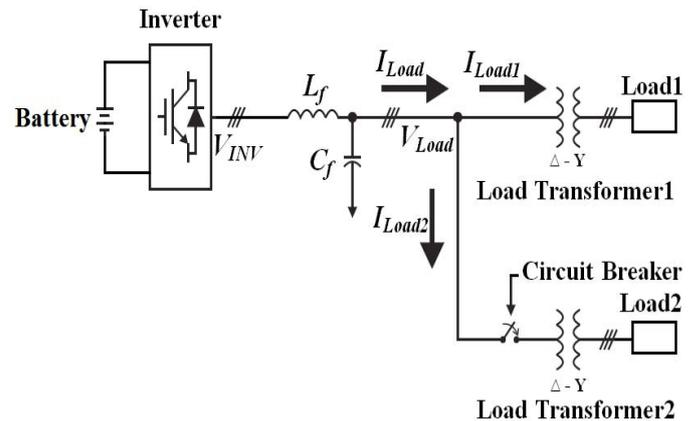
Fig. 1. One-line diagram of an on-line UPS system feeding multiple load transformers.
