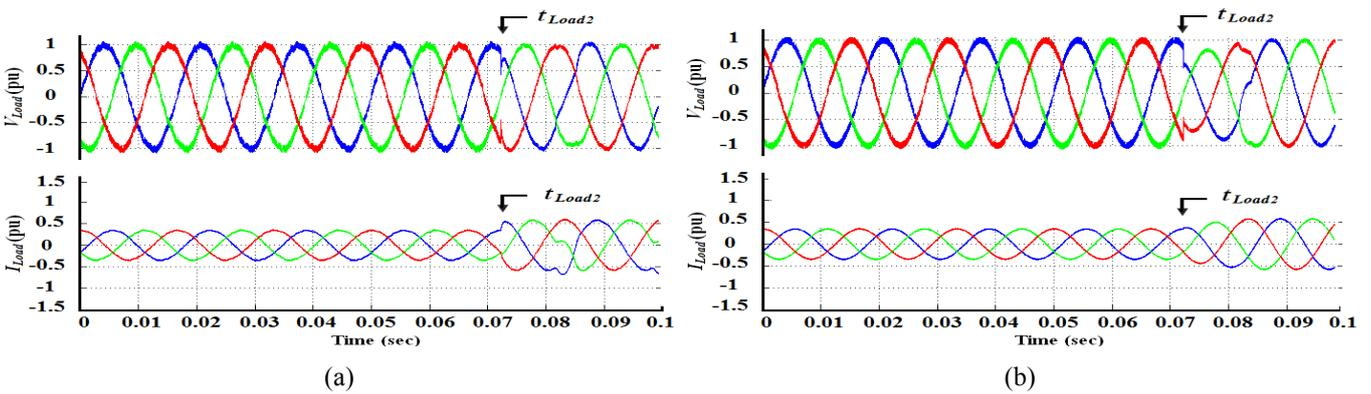
Fig. 5. Transient performance of the on-line UPS system when load transformer2 is switched in at an angle of 120 deg. of phase A. (a)  $I_{Load}$  and  $V_{Load}$  for the conventional UPS system, (b)  $I_{Load}$  and  $V_{Load}$  for the proposed UPS system.
