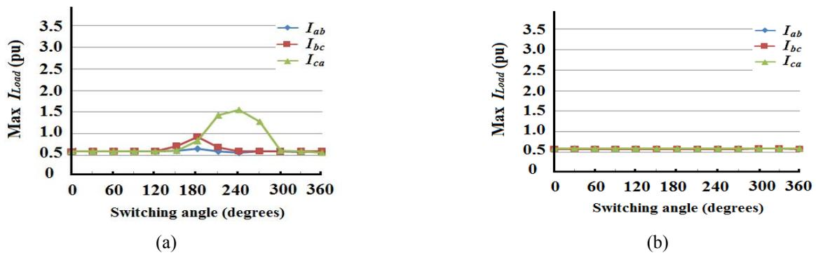
Fig. 9. Max. magnitude of  $I_{Load}$  after switching-in of load transformer2 during different switching-in angles, for the (a) conventional on-line UPS system, and (b) proposed on-line UPS system.
