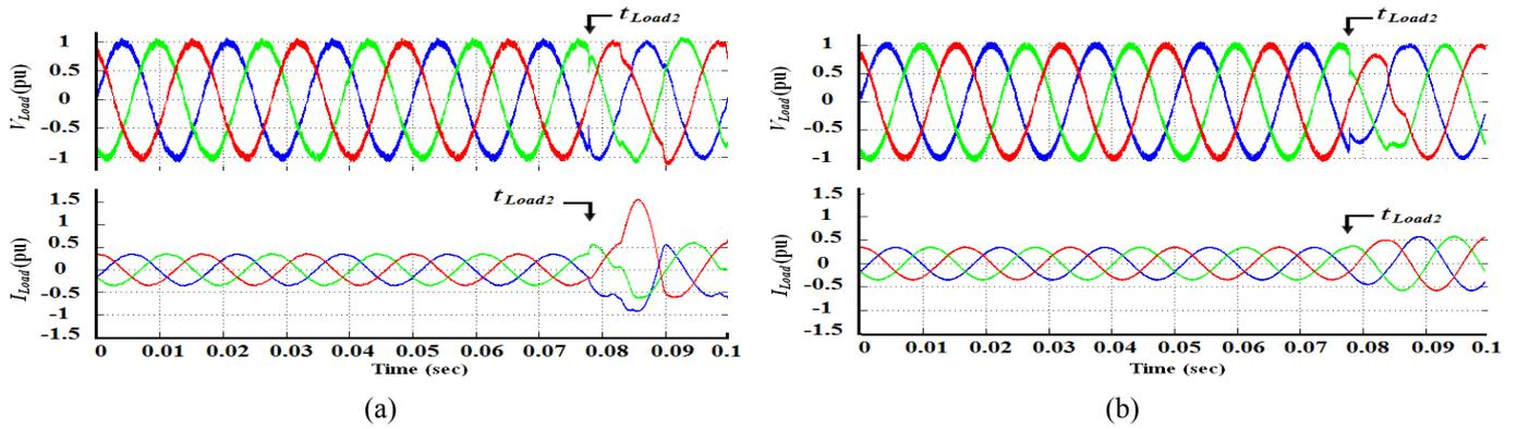
Fig. 7. Transient performance of the on-line UPS system when load transformer2 is switched in at an angle of 240 deg. of phase A. (a)  $I_{Load}$  and  $V_{Load}$  for the conventional UPS system, (b)  $I_{Load}$  and  $V_{Load}$  for the proposed UPS system.
