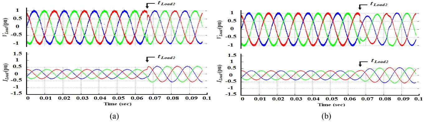
Fig. 3. Transient performance of the on-line UPS system when load transformer2 is switched in at an angle of 0 deg. of phase A. (a)  $I_{Load}$  and  $V_{Load}$  for the conventional UPS system, (b)  $I_{Load}$  and  $V_{Load}$  for the proposed UPS system.
