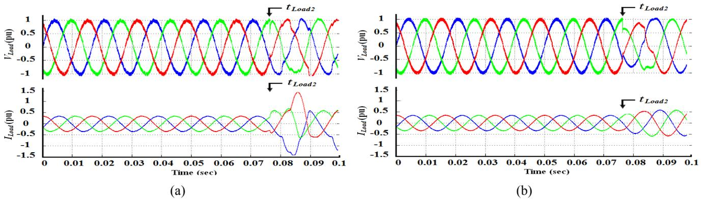
Fig. 6. Transient performance of the on-line UPS system when load transformer2 is switched in at an angle of 210 deg. of phase A. (a)  $I_{Load}$  and  $V_{Load}$  for the conventional UPS system, (b)  $I_{Load}$  and  $V_{Load}$  for the proposed UPS system.
