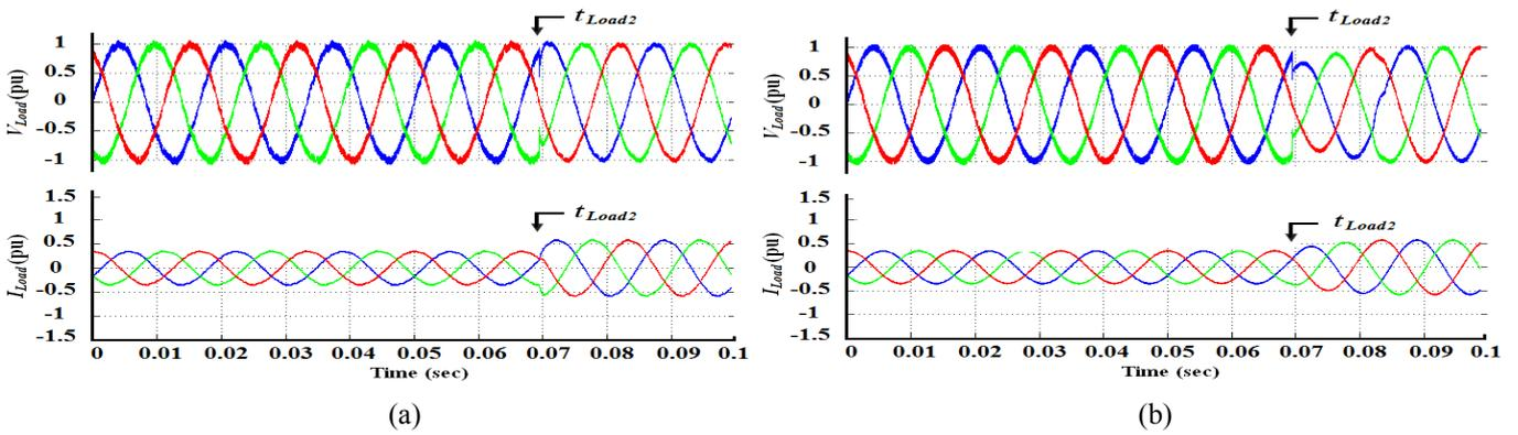
Fig. 4. Transient performance of the on-line UPS system when load transformer2 is switched in at an angle of 60 deg. of phase A. (a)  $I_{Load}$  and  $V_{Load}$  for the conventional UPS system, (b)  $I_{Load}$  and  $V_{Load}$  for the proposed UPS system.
