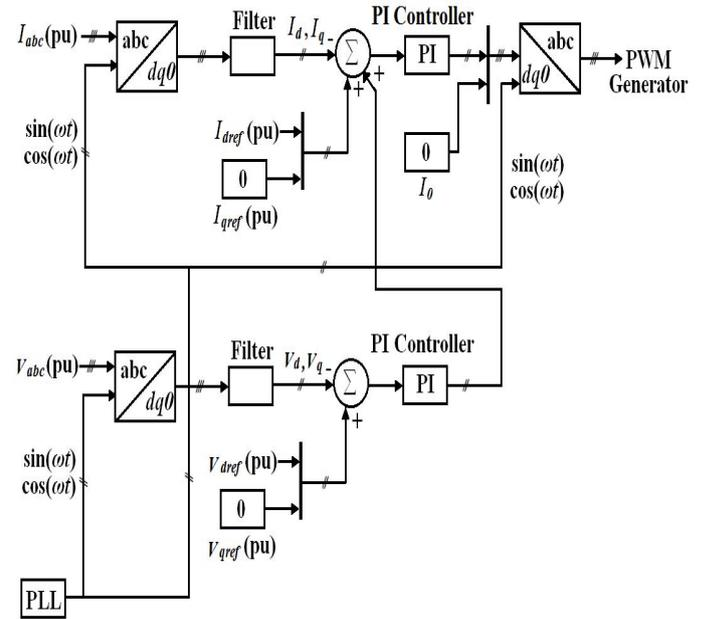
Fig. 2. Current control scheme for the inverter of the proposed on-line UPS system in  $dq0$  frame of reference.
